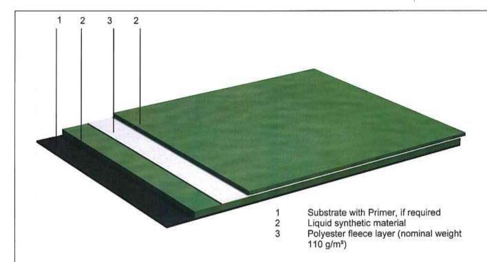
Applicable to the roof waterproofing "Triflex Towersafe":
